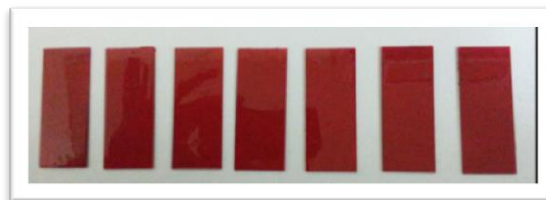
Figure 3. The image for paint red slides coated by TiO_2 -SoL then dry at room temperature for three days.
