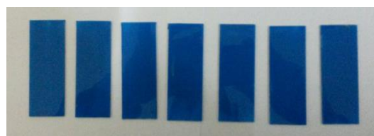
Figure 4. The image for paint blue slides coated by TiO_2 -SoL then dry at room temperature for three days.
