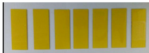
Figure 5. The image for paint yellow slides coated by TiO_2 -SoL then dry at room temperature for three days.
