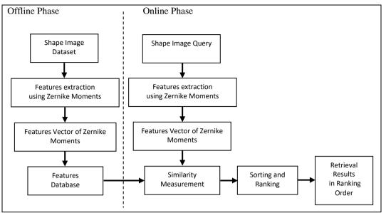
Figure 2. System Framework of the Zernike Moments Method for Image Retrieval.
