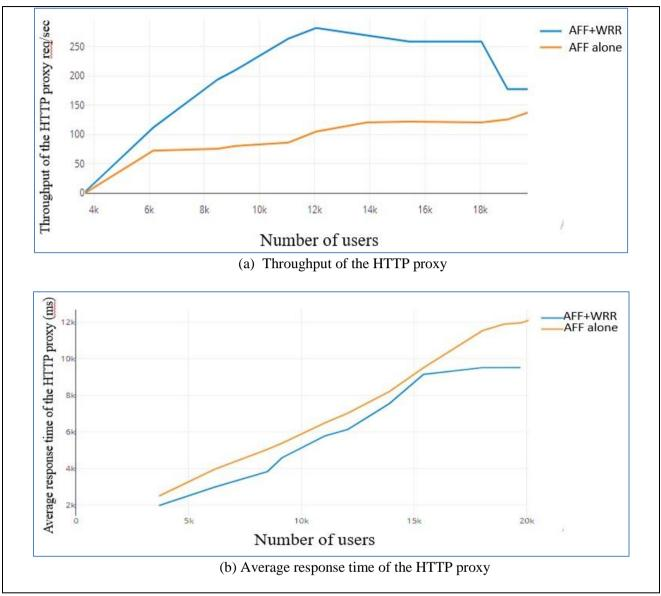
Figure 4. HTTP proxy performance comparison of the combination algorithms and AFF alone
