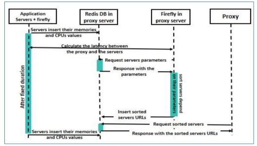
Figure 3. The sequence diagram of load balancer procedure
