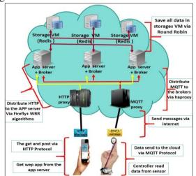
Figure 2. Architecture of IoT cloud computing system
