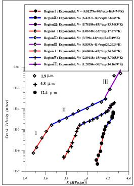
Fig (5) explains fitting the experimental data of (V-K)plot with exponential function of alumina ceramics .
