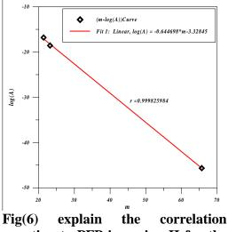
Fig(6) explain the correlation equation to PFP in region II for the alumina ceramics.
