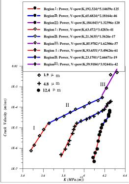
Fig (4) explains fitting the experimental data of (V-K)plot with Paris function of alumina ceramics .
