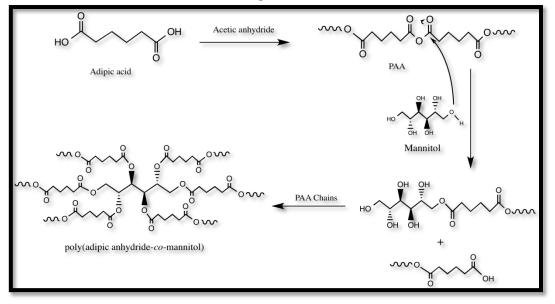
Scheme 2. Crosslinking mechanism of poly(adipic anhydride-co-mannitol).
