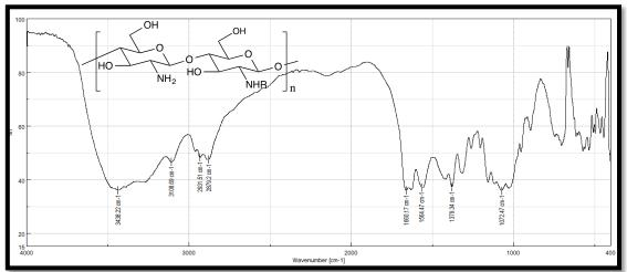
Figure 1. FT-IR spectrum for chitosan
