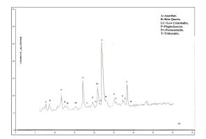
Fig. 8: X-Ray Diagram of ceramic disc filter.
