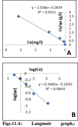
Figs.11.A: Langmuir graph,: Frundlich graph of data for adsorption capacity of Co.
