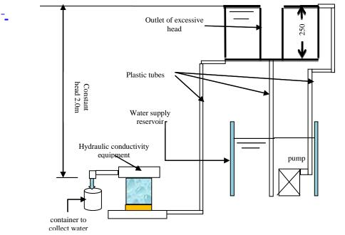
Fig.7. Schematic diagram of hydraulic conductivity test rig.
