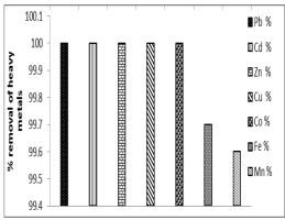
Fig 9: % of removal of heavy metals at concentration 1mg/l.
