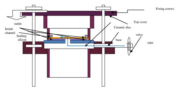
Fig. 5. Schematic diagram of hydraulic conductivity test equipment.
