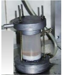
Fig. 4. General view of hydraulic conductivity test equipment.
