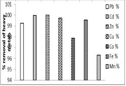
Fig 10: % of removal of heavy metals at concentration 10*mg/l*.
