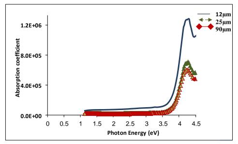
Fig. 4 Absorption coefficient with photon energy
