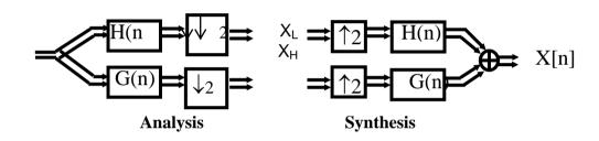
Fig. 2 Analysis and synthesis of input signal using multiwavelet transform
