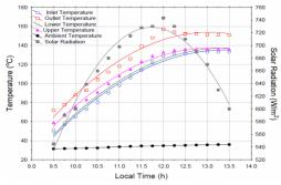
Fig (5) Total solar radiation and temperatures history of PTSC
