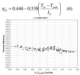
Fig (8) Thermal efficiency curve of the collector
