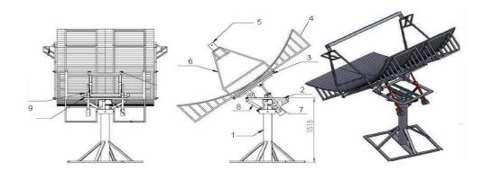
Fig (1) The schematic of PTSC (1) Axial Motion Guide Ass. (2) Tilting Motion Base (3) Tilting Motion Ass. (4) Reflecting Ass. (5) Thermal Receiver Ass. (6) Heat Receiver Support (7) DC actuator motor (8) Side Support Angle (9) Bracate  $\emptyset$  50.
