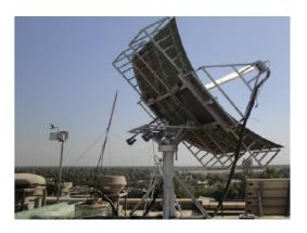
Fig. (4) Photographic of PTSC setup
