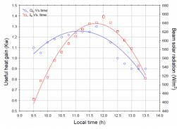
Fig (6) Variation of beam radiation and useful heat gain with time
