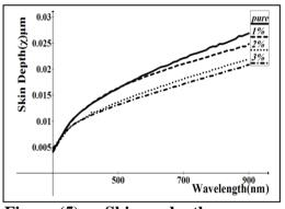
Fig. (5) Skin depth versus wavelength for the as deposited films.
