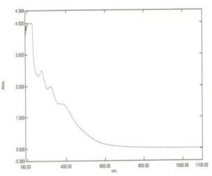
Figure 4. UV–vis spectrum showing absorption of  $(10^{-4} \text{ M})$  aqueous solution of silver nitrate with *M.parviflora* extract
