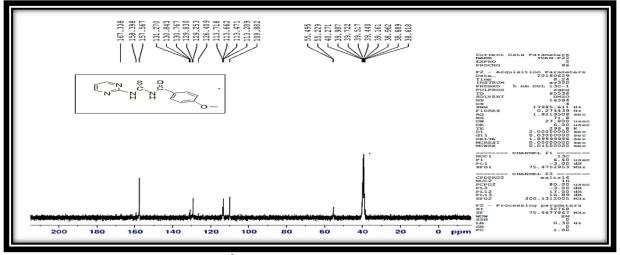
Figure 3. <sup>1</sup>H-NMR spectrum of ligand(MPB).
