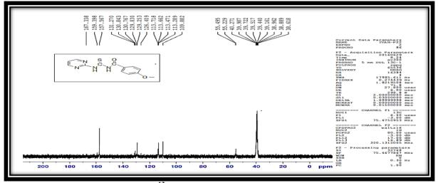
Figure 4.<sup>13</sup>C -NMR spectrum of ligand(MPB).
