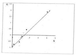
Fig. (1): Determination of the reactivity ratios for AM / AA system at 70°C Finemon – Ross plot . where G=(F-1)f/F,  $X = f^2/F$
