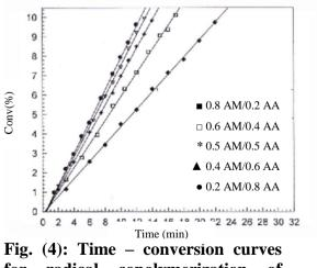
for radical copolymerization of AM/AA system
