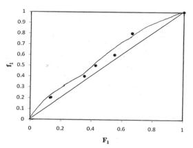
Fig. (3): Coploymer composition curves. Experimental data are represented by (•) – AM/AA System.
