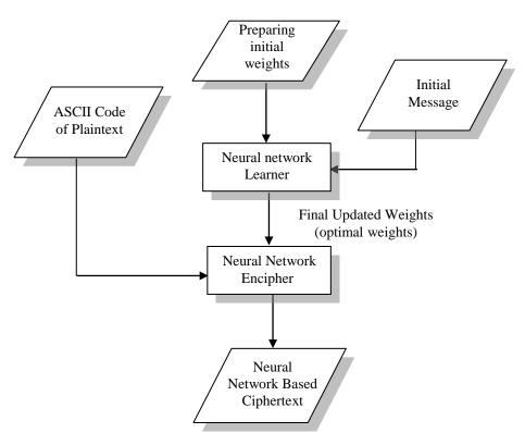
Fig 5: A Block diagram of NNBCEM
