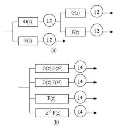
Fig. (1) Two-scale iterated filter bank and an equivalent structure
