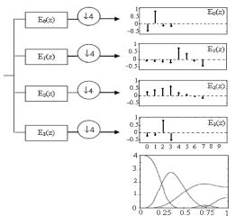
Fig. (2) Two-scale filter bank structure using the slantlet
