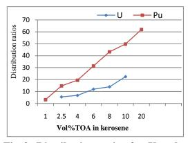
Fig 3: Distribution ratios for U and Pu from 2.5M HNO3 and as a function of amine concentration
