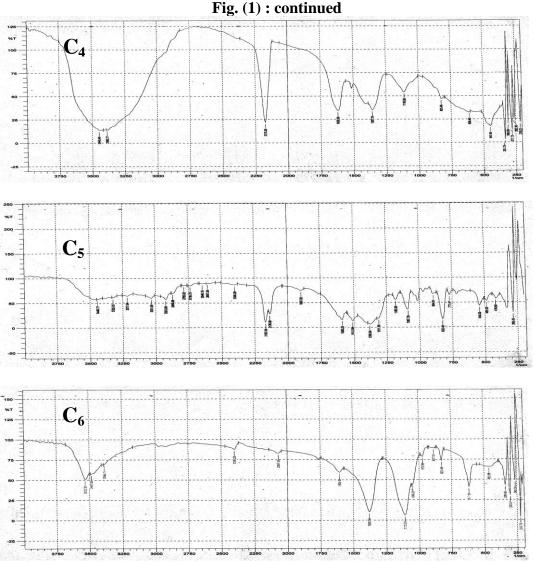
FTIR Spectra of HL<sub>II</sub> complexes C<sub>4</sub> of Co(II) ; C<sub>5</sub> of Cu(II) and C<sub>6</sub> of Cd(II)
