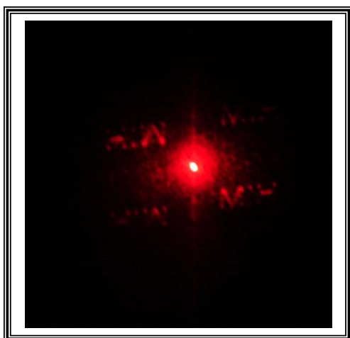
Fig(7): optical reconstruction image of a hologram with random phase.
