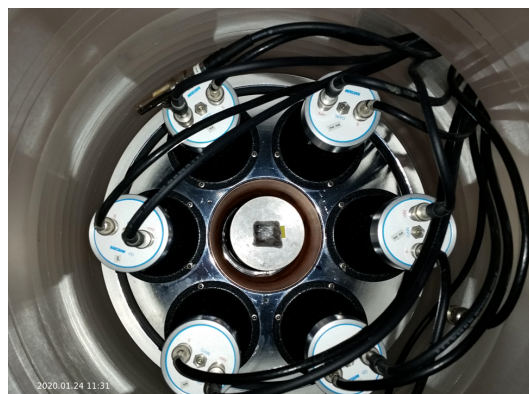
Figure 2: GEM90 HPGe detector surrounded by the NaI(Tl) annulus. The F2 specimen is placed on the top of the germanium crystal. The six photomultiplier tubes on the top of the NaI annulus are also visible.
