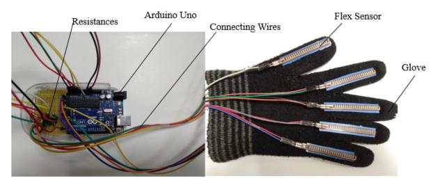
**Figure 2.** Flex sensor, gyroscope, and Arduino-based data glove designed for capturing ASL-based gestures.
