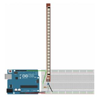
Figure 3. A simple interconnection of the flex sensor with the Arduino microcontroller.
