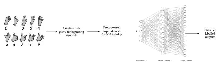
Figure 1. An overview of complete methodology for NN-based ASL recognition.
