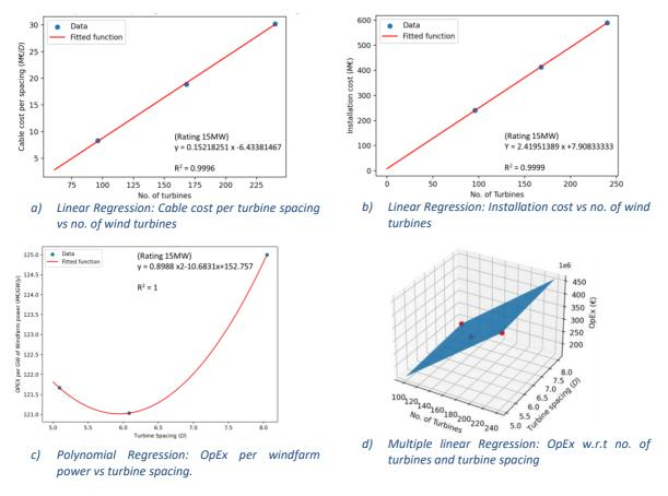
Figure 5.10 ECN cost extrapolation using regression methods<sup>8</sup>
