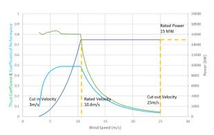
Fig. 11. Coefficient of Performance, Thrust coefficient and Power for NREL 15MW wind turbine
