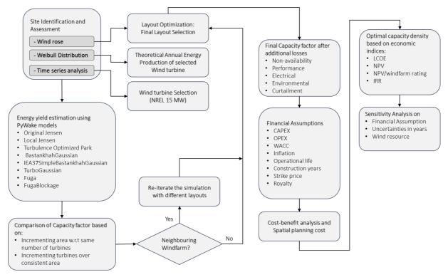
Figure 5.1 Flowchart of procedure for identifying optimal capacity density<sup>3</sup>
