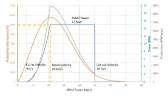
Fig. 2. Power curve, weibull curve and theoretical annual production
