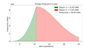
Fig. 12. Annual energy production for the average value of shape and scale factor  $% \left( {{{\left[ {{{\rm{T}}_{\rm{T}}} \right]}}} \right)$
