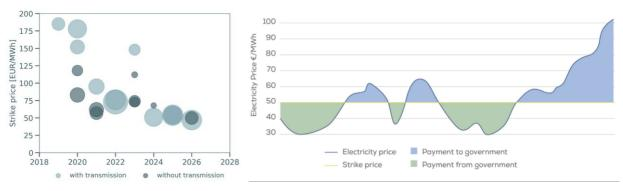
Figure 4.2 Strike price values for offshore wind<br/>in recent auction [21]Figure 4.3 Revenue stabilization from two-sided Contract for Difference<br/>[22],[23]
