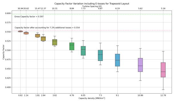
Figure 5.9 Box plot for net capacity factor variation using Trapezoidal layout
