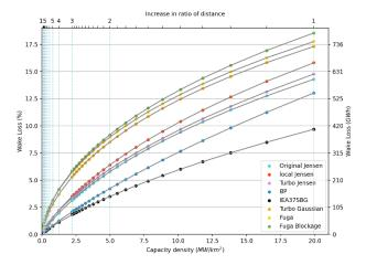
Fig. 5. Wakeloss vs Capacity density/Scaled ratio for different wake models
