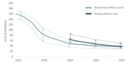
Figure 4.5 Projection for LCOE of offshore wind energy [21]
