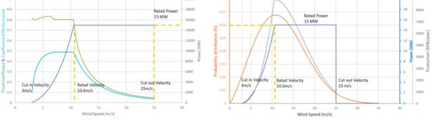
*Figure 3.12 Figure. Power curve, Coefficient of thrust and performance*
