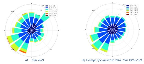
Figure 3.7 Wind rose at height 160m for the selected site
