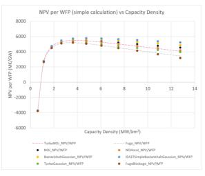
d) NPV per WFP vs Capacity Density (simple method)
