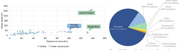
Figure 3.5 Water depth and shore locations of wind turbines installed till date<sup>1</sup> [4]
