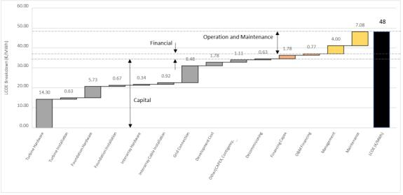
Figure 6.7 LCOE breakdown according to tuned parameters
