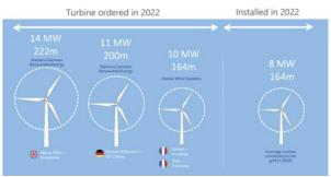
Figure 3.2 Yearly average of newly- installed offshore wind turbine rated capacity (MW)[4]
