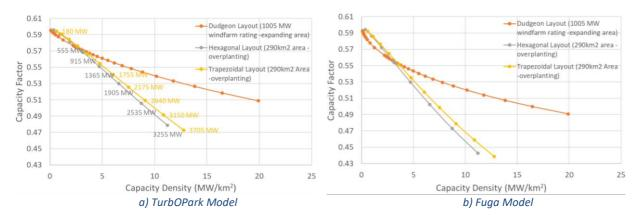
Figure 5.4 Capacity Factor Comparison based on industry-standard wake models<sup>5</sup>
