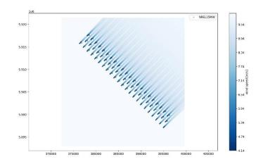
Fig. 16. Flowmap of NREL 15MW WT placed in Dudgeon layout
