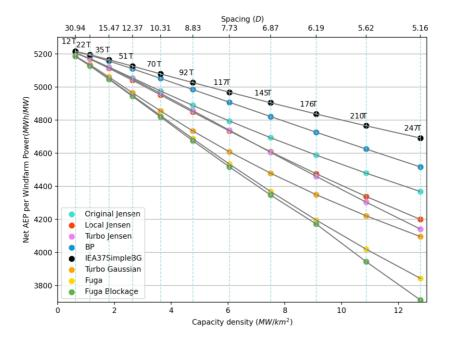
Figure 5.7 AEP<sub>ne</sub>t /WFP vs Capacity density
