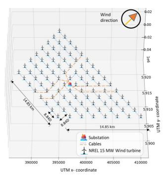
Figure 7.1 3D view of the wind farm on the proposed site with capacity density of 4.76 MW/km<sup>2</sup>
