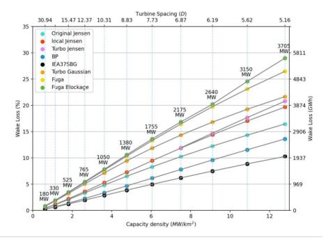
Figure 5.8 Wake loss vs Capacity density
