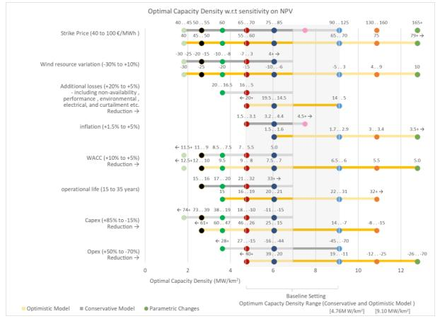
Figure 6.11 Optimal capacity density from NPV sensitivity analysis
