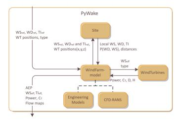
Fig. 15. Flowchart of PyWake simulation
