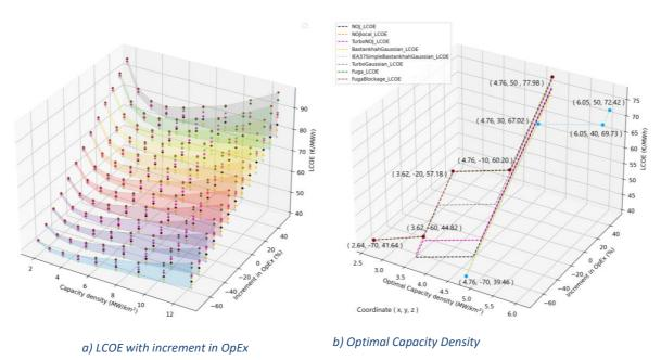
Figure 6.9 LCOE sensitivity with respect to OpEx
