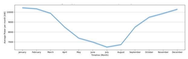
Figure 3.11 Predicted average hourly production for each month within the span of 32 years
