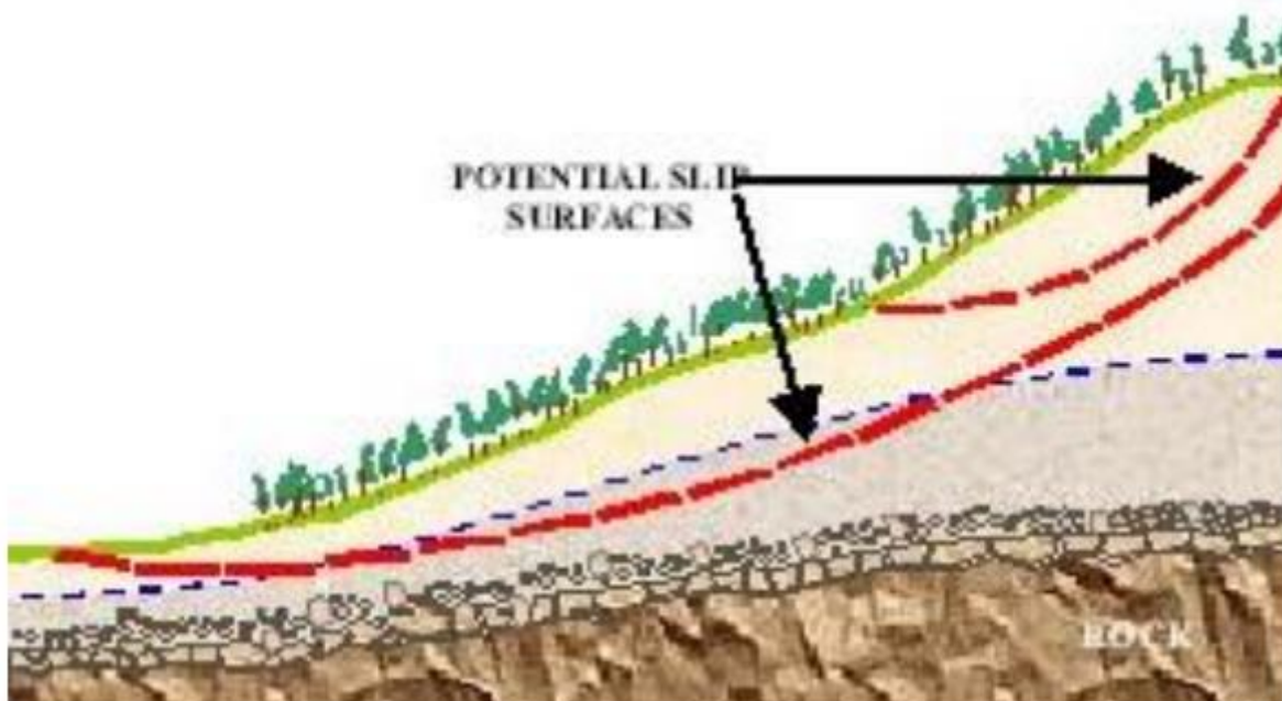
Figure 3.45 potential slip surface (Gue and Fong 2003) [41]
