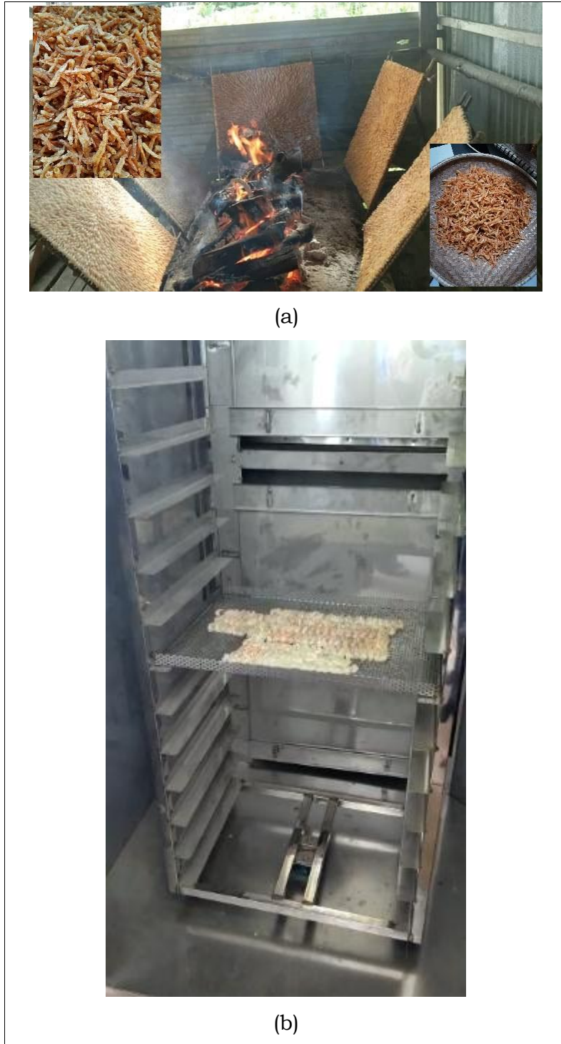
Gambarajah 1: Pemprosesan sesar unjur (a) tradisional (b) mesin salai bertenaga solar
