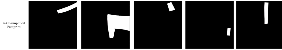
Fig. 6. Regularized building footprints after applying the GAN-based regularization method to map objects shown in bottom row of Fig.5. The Poly -GAN architecture learns to reshape the irregular building footprints while preserving the overall shape of the building and other important features such as corners.
