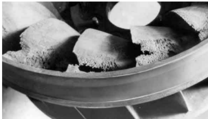
Figure 1.9: Cavitation damage to the blades of a Francis turbine [3]
