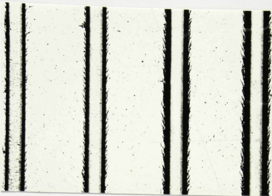
Obr.25 Scratches test na povlaku ZrN_{40} - 60x
