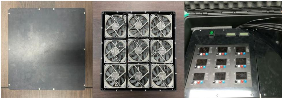
Fig. 11. A portable large-area blackbody frontal panel(left), cooling fan in the back(middle), and temperature controller(right).
