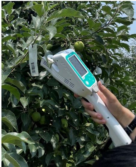
Fig. 9. Stomatal conductance measurement using porometer (LI-600P, LI-COR, USA).
