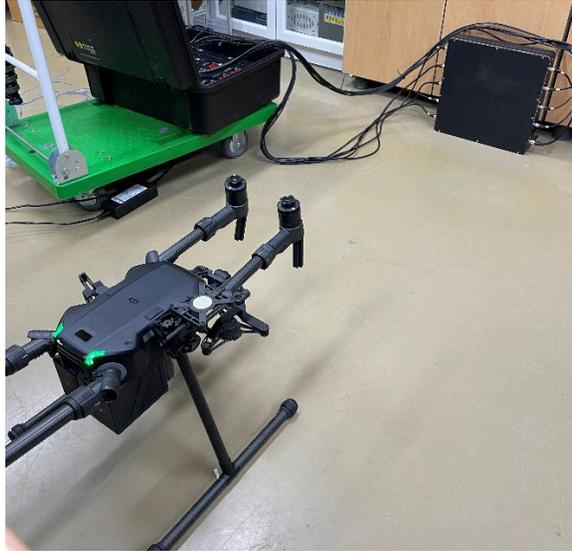
Fig. 12. An indoor performance evaluation of the portable, large-area blackbody system.
