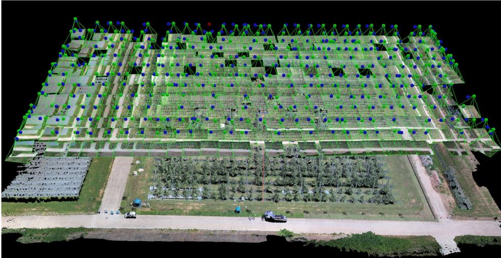
Fig. 18. Aerial images from each camera position (blue points) and calibrated position (green points) (13th July, 2021).
