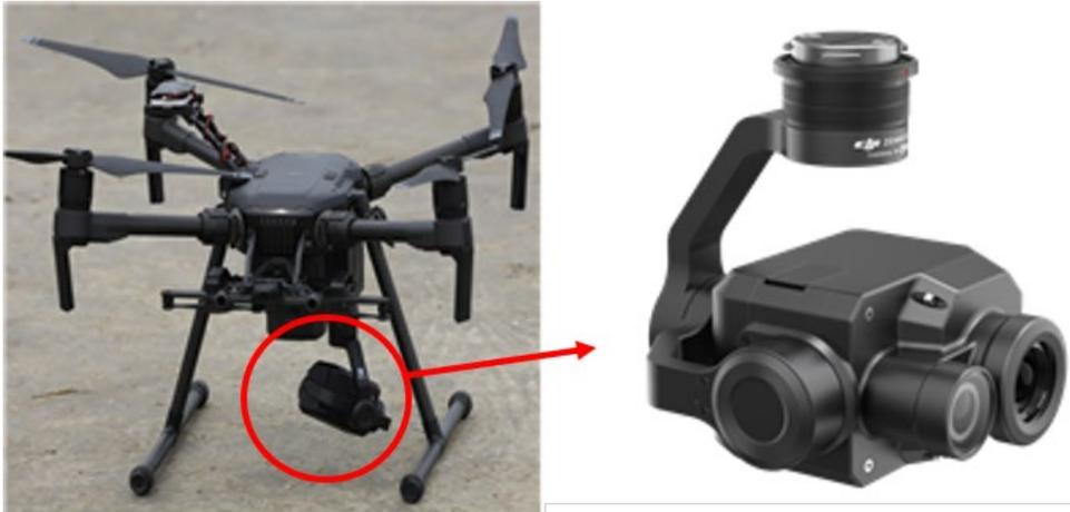
Fig. 10. Thermal imaging sensor (Zenmuse XT2, FLIR Systems Inc., USA) loaded on the UAV.
