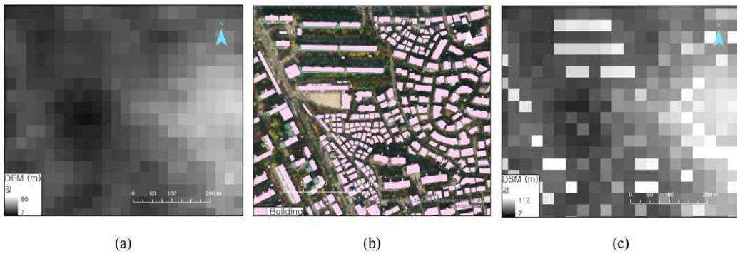
Figure 3-4. Process for DSM. (a) ASTER GDEM (Basic DEM) (b) building polygon (c) DSM made by adding height of rasterized (b) to (a)
