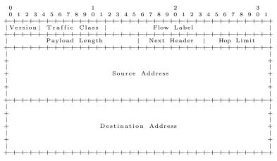
Listing 2.2: IPv6 header according to RFC8200
