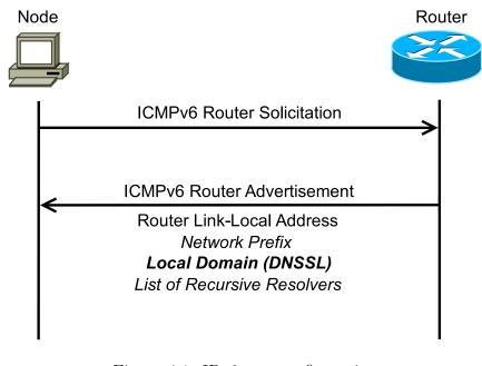
Figure 4.1: IPv6 autoconfiguration
