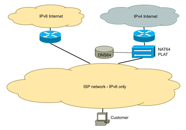
Figure 2.6: NAT64/DNS64 network with IPv6 only customers
