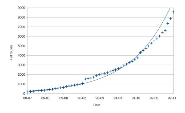
Figure 2.3: Number of IPv4 routes before CIDR (source: RFC1519[27])
