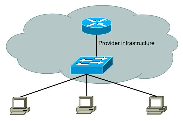
Figure 4.5: Example of flat designed network
