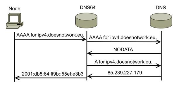
Figure 2.9: DNS64 principle of operation
