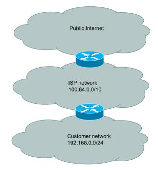
Figure 2.4: Typical deployment of NAT44 in residential customer environment
