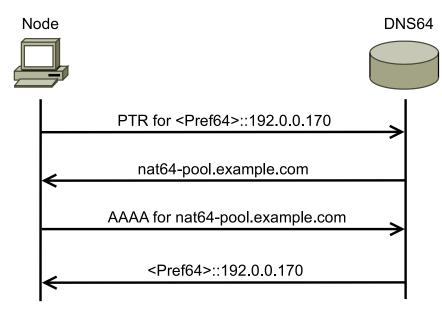
Figure 3.2: Validation of NAT64 prefix according to RFC 7050[1]
