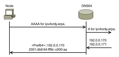
Figure 3.1: Detection of NAT64 prefix according to RFC 7050[1]
