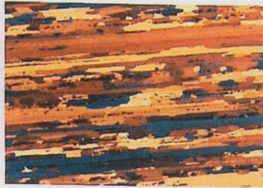
Fig. 5-26. The partially recrystallized structure of a bar 36 mm in diameter made of AlZn6MgCu1.5 alloy. The photograph shows the annulus area of the bar with fine bands of the non-recrystallized structure ( \times 50 ).
