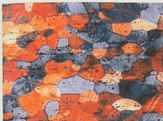
Fig. 5-32. Twinning of grains in AlMg5 alloy ( \times 100 ).
