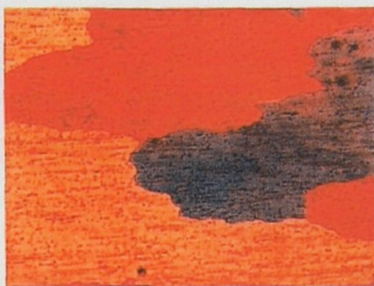
Fig. 5-33. Coarse grains in the entire cross-section of Al99.5 alloy ( \times 100 ).
