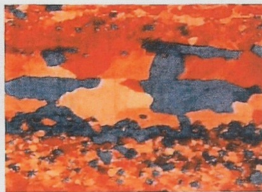
Fig. 5-34. The necklace condition of the grains in Al 99.5 alloy ( \times 65 ).
