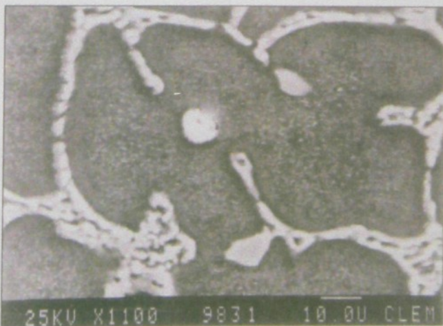
OBR. 4. Samostatná Pb-fáza globulitickej morfológie - zv. 850x FIG. 4. Individual Pb-phase of the globular shape morphology - magnification 850x
