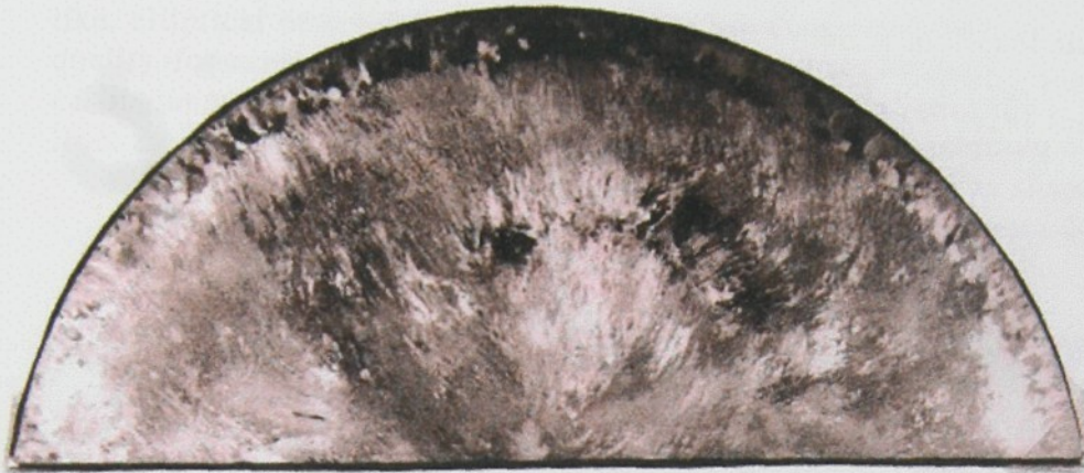
Fig. 5-5. Macrostructure of a shaft with a feather-like structure in AlMgSi0.5 on more than 50% of the area (reduced \times 1.5 ).
