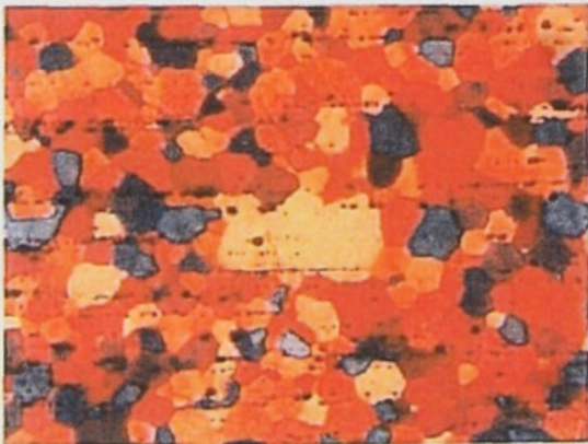
Fig. 5-30. The wide-scale condition in AlMg5 alloy. In the grains with a size of 40–50 \mu\text{m} there are grains with a size of 120–130 \mu\text{m} ( \times 100 ).
