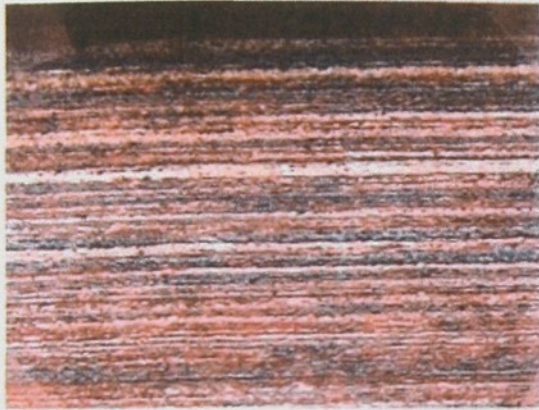
Fig. 5-8. Microstructure of the non-recrystallized fine fibrous structure at the edge of a pipe of AlMg2Zn alloy ( \times 100 ).
