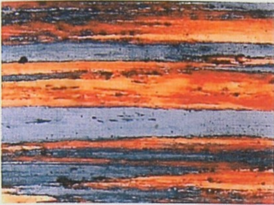
Fig. 5-12. Microstructure of thicker fibres of the non-recrystallized structure in a bar 35.5 mm in diameter made of AlZn6.5Cu1.5Mg alloy ( \times 100 ).
