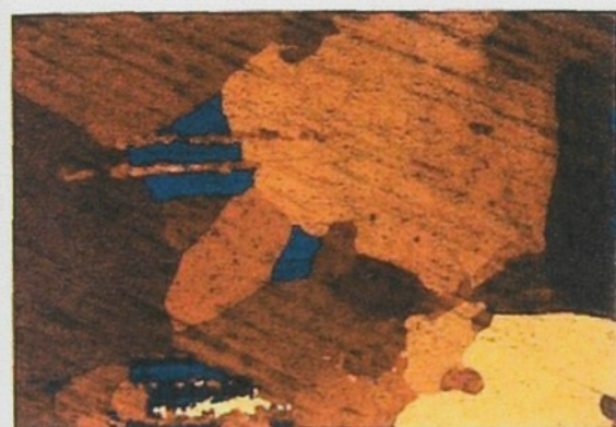
Fig. 5-34. The necklace condition of the grains in Al 99.5 alloy ( \times 65 ).
