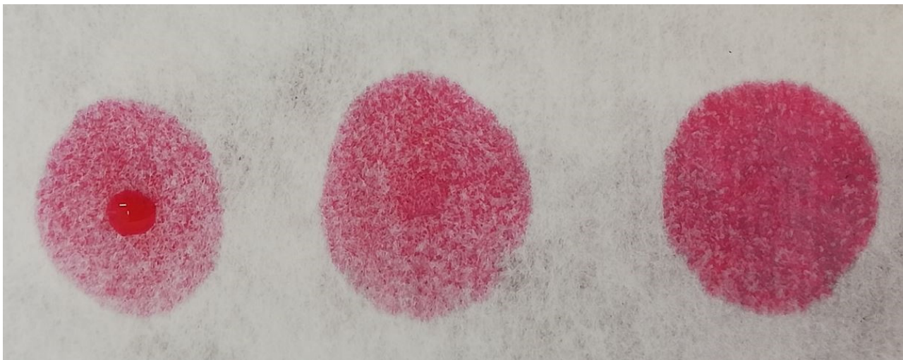
Figure 18. Three samples made at a time interval of 10 s on paper with surface hydrophobization using a spray-applied hydrophobic varnish: left with incipient surface absorption, middle with visible hydrophobic defects, right almost absorbed.
