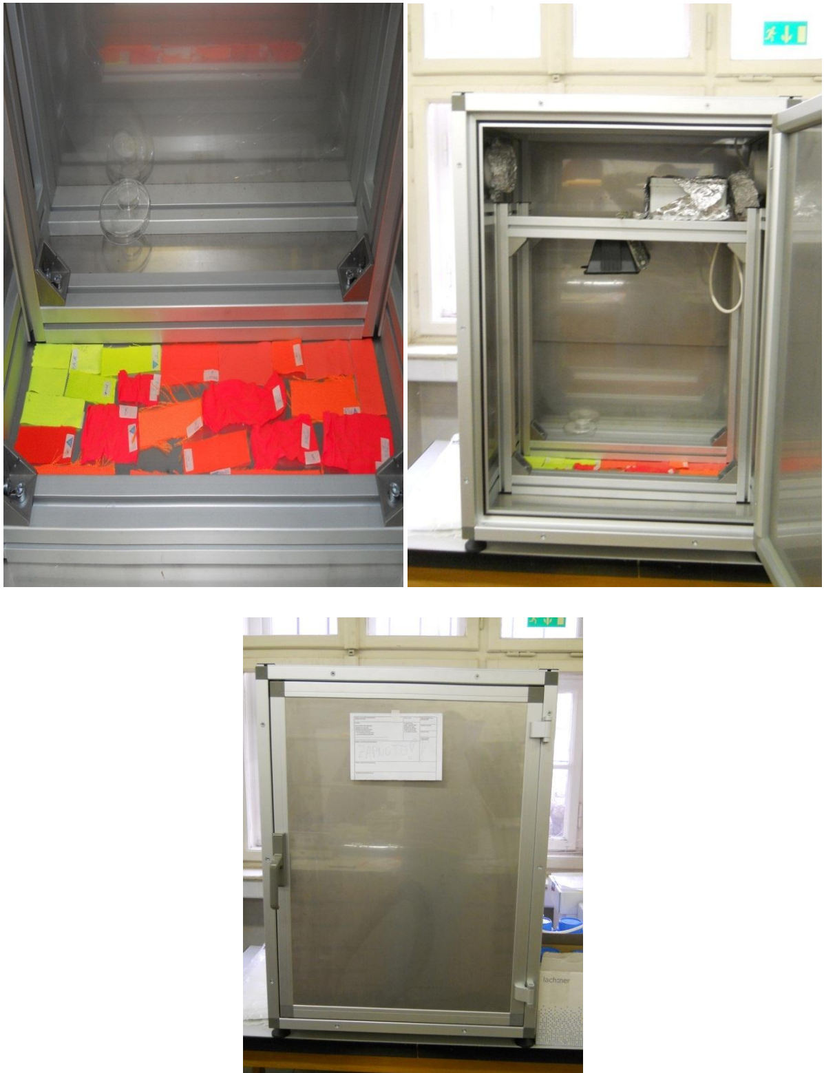
Fig. 3-5: Laboratory pictures of the whole light exposure equipment/set up.
