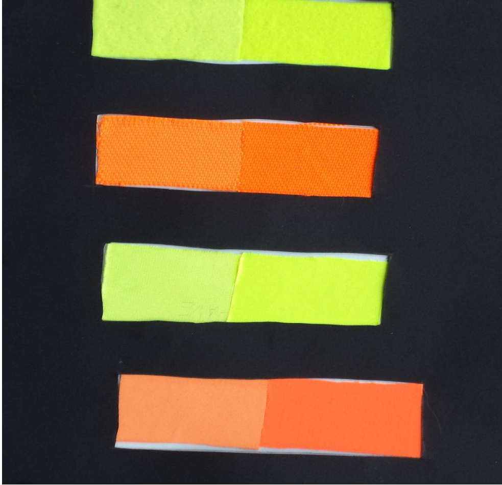
Fig. 4-1 A photograph showing visual inspection of samples. Comparison of UV exposed samples (left) and unexposed samples (right).
