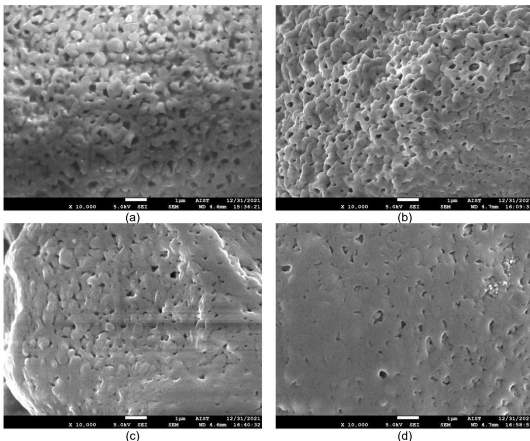
**Figure 5** SEM images of the microcapsule polymer shell after the fabric treatment (a) M1 microcapsules (0.15 g of cinnamon oil); (b) M2 microcapsules (0.25 g of cinnamon oil); (c) M3 microcapsules (0.35 g of cinnamon oil); (d) M4 microcapsules (0.45 g of cinnamon oil)
