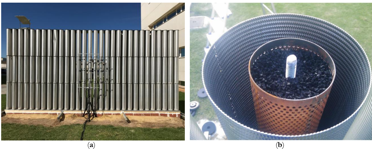
Figure 45. Sonic crystal (SC) barrier sample implemented on the campus of Universitat Politècnica de València: (a) Appearance of SC barrier sample made of three rows of absorbing cylindrical units, along with experimental setup; (b) internal cross-section of a cylindrical unit, consisting of a porous core made of rubber crumb and outer micro-perforated aluminium shell [34].
