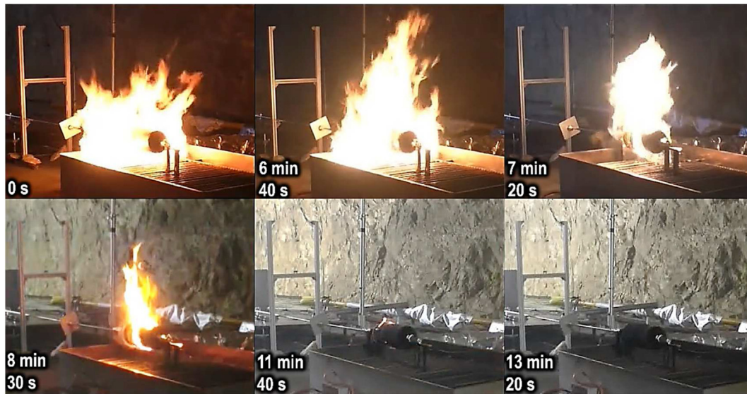
Fig. 5 – Snapshots of the \mu LNB tank fire test with COPV#CB-1.
