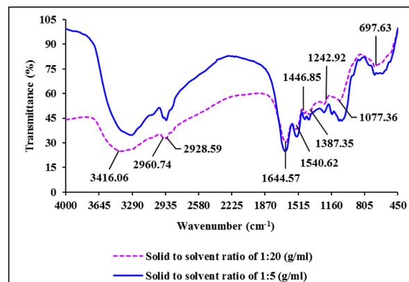
**Fig. 3.** FTIR spectra of SMPI in the solid to solvent ratio of 1:5 (g/mL) and 1:20 (g/mL).
