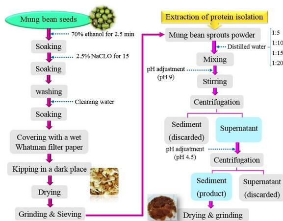
**Fig. 1.** Schematic process diagram of the overall experimental design.
