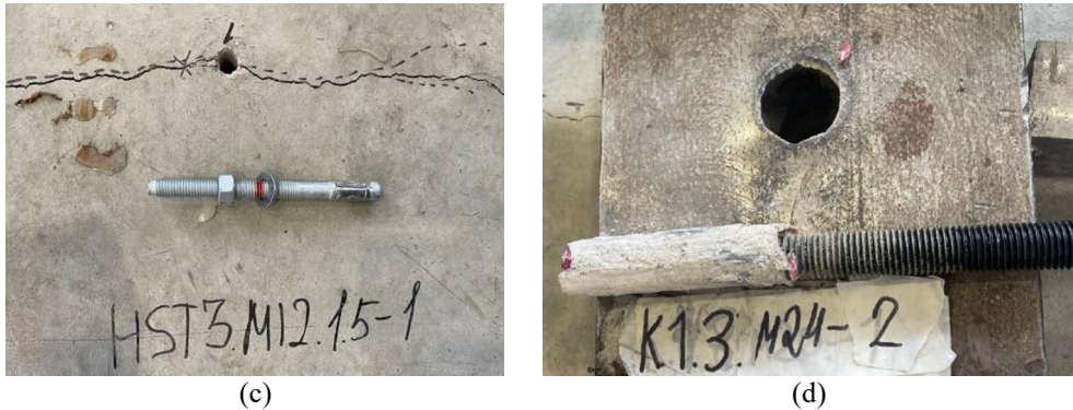
Fig. 2. Failure mechanisms for anchorages: a) steel failure; b) concrete cone failure; c) pullout failure; d) bond failure
