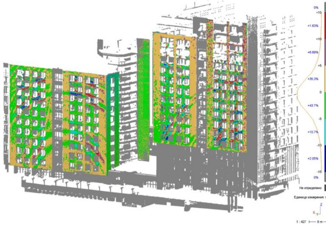
Fig. 4. Determination of the initial rolls of the building based on the results of laser scanning
