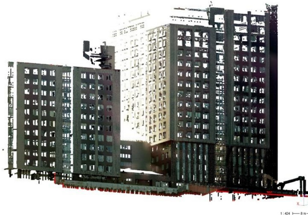
Fig. 3. The result of scanning the building structures scanning total station Leica MS60
