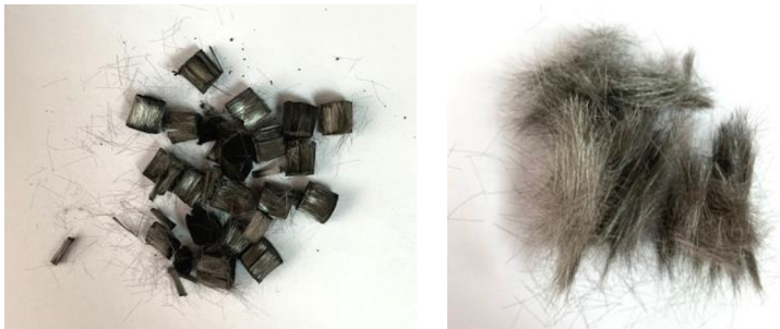
Fig. 1. Fiber from an amorphous ferromagnetic alloy in a glass borosilicate sheath in a glued (a) and separated (b) form.
