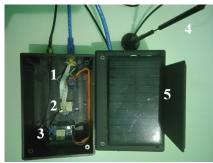
Fig. 7. Node (LoRa-Tx); (1) Board Arduino nano, (2) LoRa RA-02, (3) GPS UBlox Neo 6M, (4) Antena, (5) mini solar cell with modul charger and battery.
