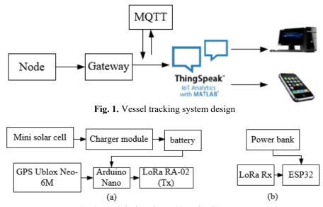
Fig. 2. Tool design chart: (a) node; (b) gateway
