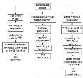
Fig. 6. Experimental testing chart
