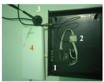
Fig. 8. Gateway (LoRa-Rx); (1) ESP32, (2) LoRa RA-02, (3) Antenna, (4) Powerbank.
