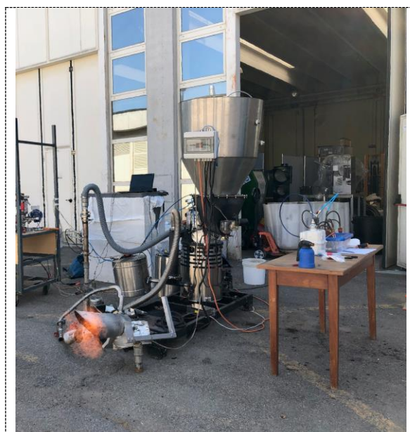
Figure 7. PP30 prototype during the gasification efficiency test.
