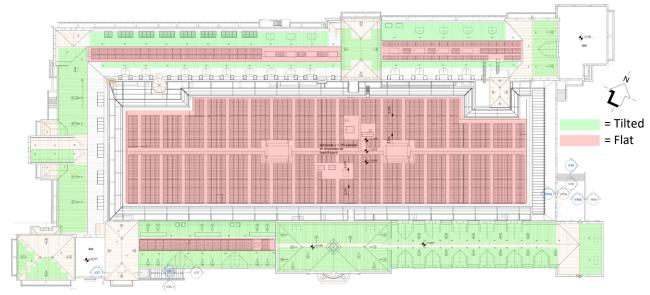
Figure 27 Overview of solar collector layout (Source of original drawing is design document of Mijnbouwstraat)
