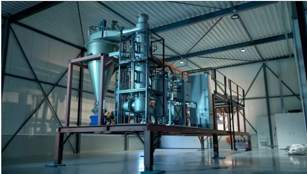
Figure 42: First experimental metal fuels combustion system, for iron fuel regeneration process. Photo is adopted from [17]
