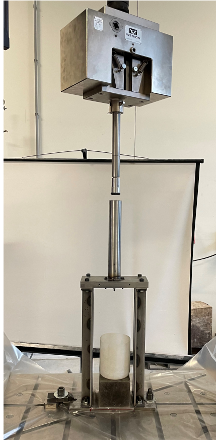
Figure 3.12: Test setup of RAM Extruder.
