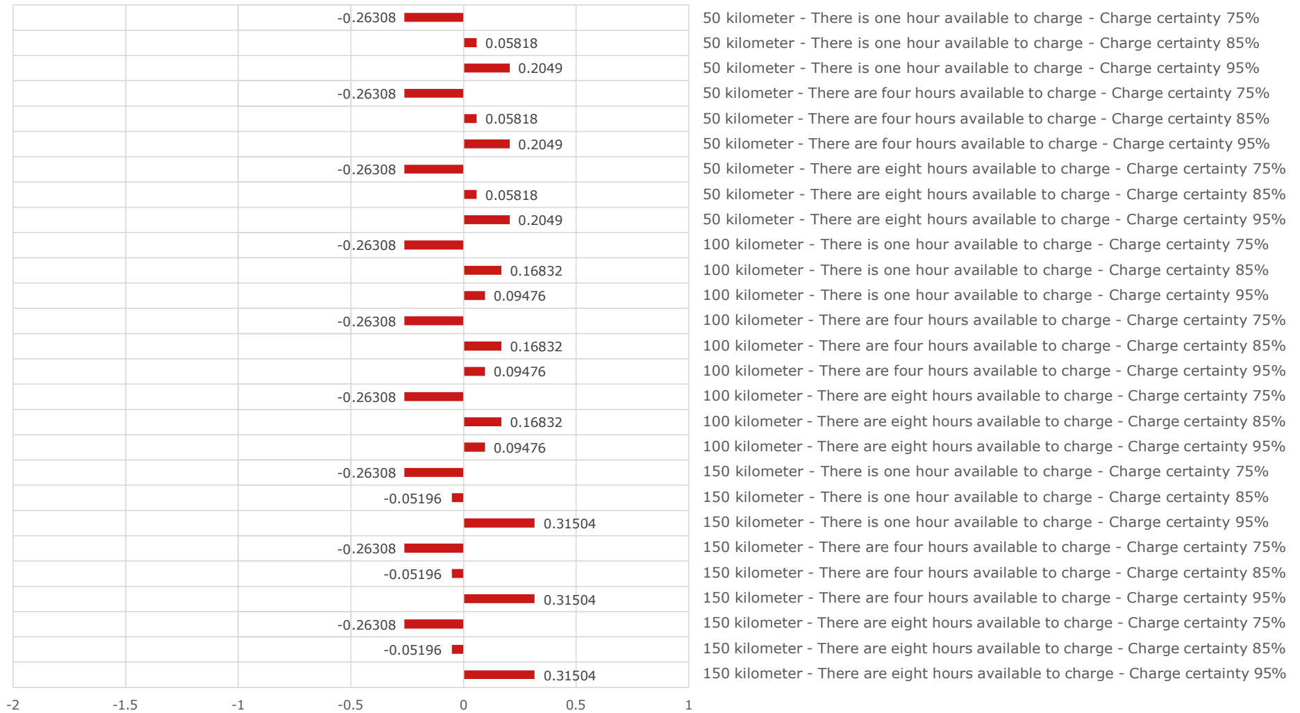
Figure 31. MNL path-worth utility of context effect for charge certainty of the reduced MNL model before excluding several context effects
