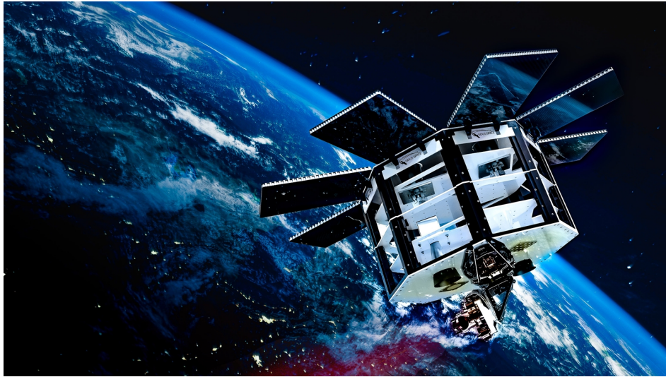
Figure 1.2: Optical satellite communication is becoming an important solution to achieve safe and high-speed communication. This image showcases a high-efficiency miniature demonstrator for optical satellite communication that is being developed by TNO [7].
