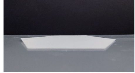
Figure 24: Warpage in print 16, printed with a laser power of 6.90 W and bed temperature of 169 °C.
