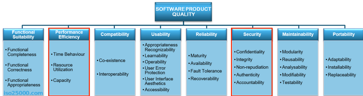
Figure 2.2: Quality model for software products by ISO/IEC 25000 [42]. The quality indicators that will be used for the evaluation of the final approach of the QOC are indicated by a red border.
