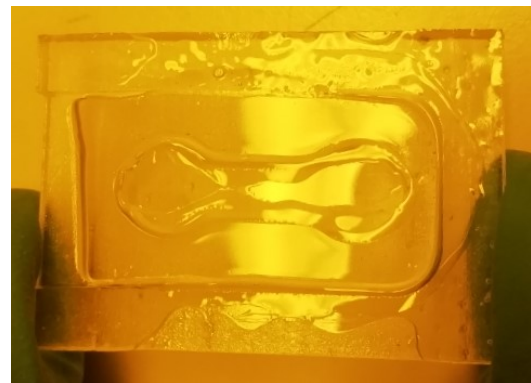
Figure 4.33: After curing the PDMS the NOA81 was still mostly a liquid
