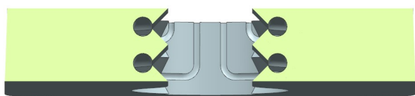
Figure 4.18: Cross section PDMS part with circular nutrient channels
