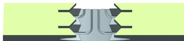
Figure 4.19: Cross section PDMS part with rectangular nutrient channels
