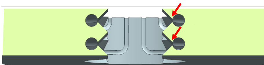
Figure 4.20: Red arrows indicating locations where the air gets stuck
