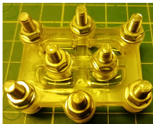
Figure 4.43: Mold for upside down filling assembled
