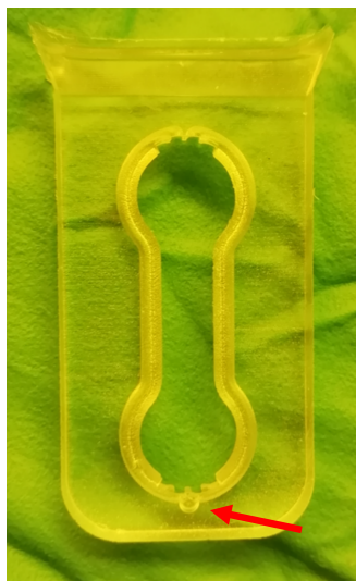
Figure 4.39: Piece of PDMS turned out well, except for the air bubble (red arrow)
