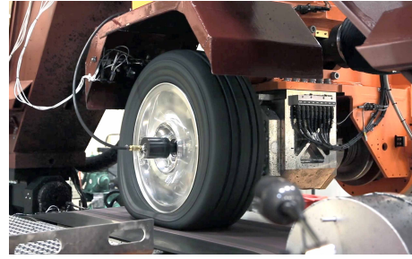
Figure 2.2: MTS Flat-Trac ® Tire Force & Moment Measurement system [10].
