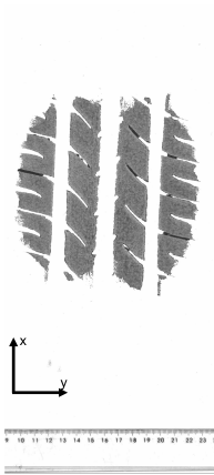
Figure G.2: Contact patch measurement for F_z = 3700 .
