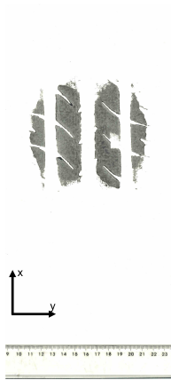
Figure G.1: Contact patch measurement for F_z = 1850 .
